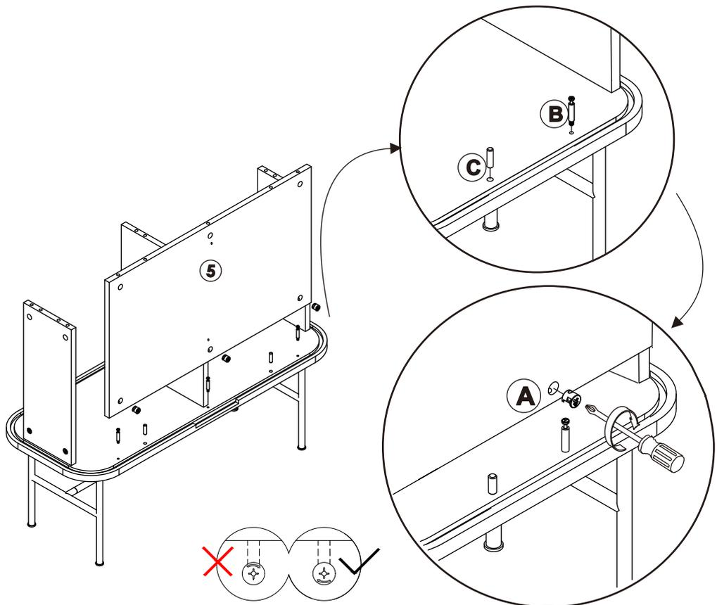
Use Minifix Housing(A), Minifix Bolt(B) and Wood Dowel(C) to connect Back Panel (5) with unit together with screw driver (not included).
