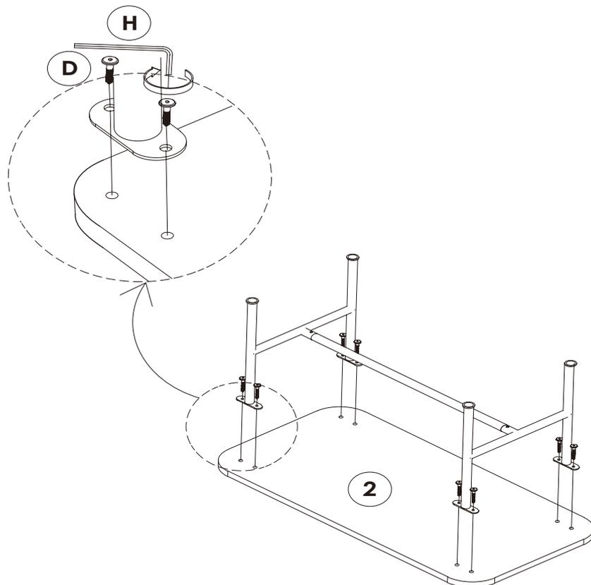
Place Metal Leg Assy onto Bottom Panel (2). Tighten the JCBC screw (D) by using Allen Key (H)
