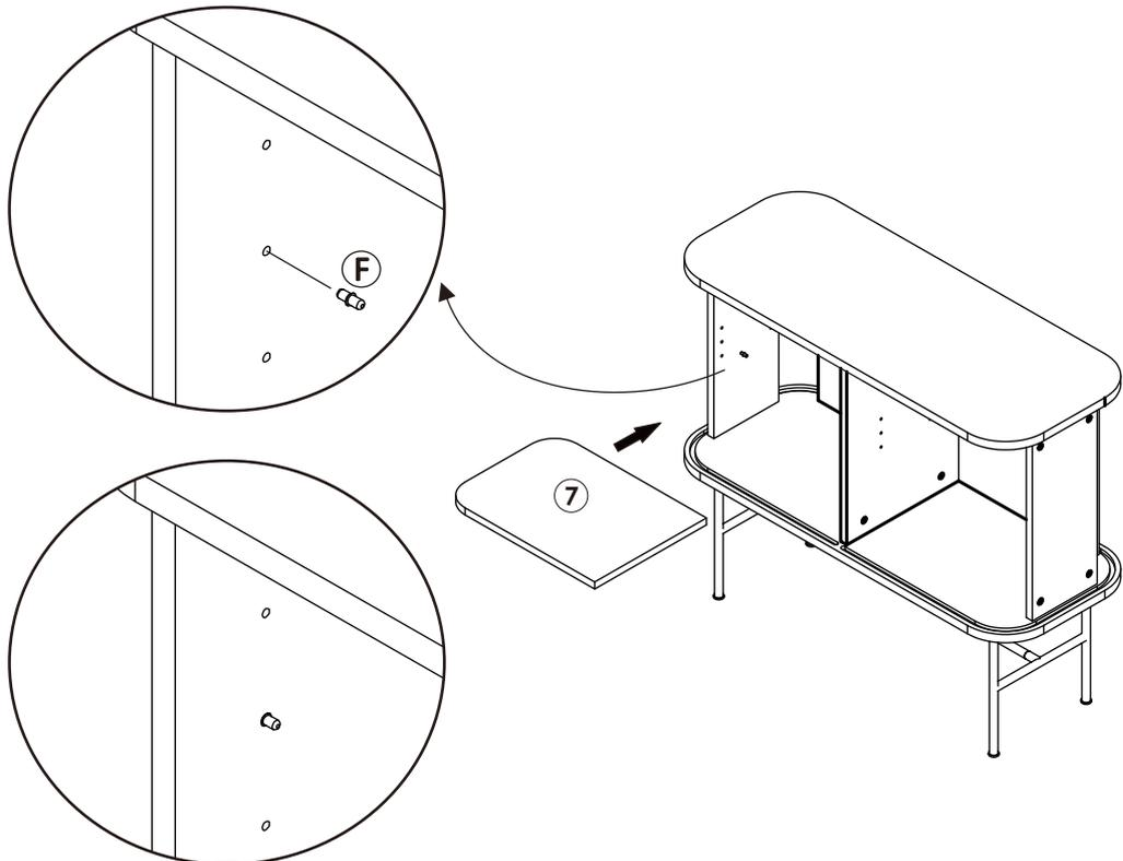
Insert Shelf Pin(F) into Side Panel and Center Panel.Place adjustable shelf panel(7) into inside unit.
