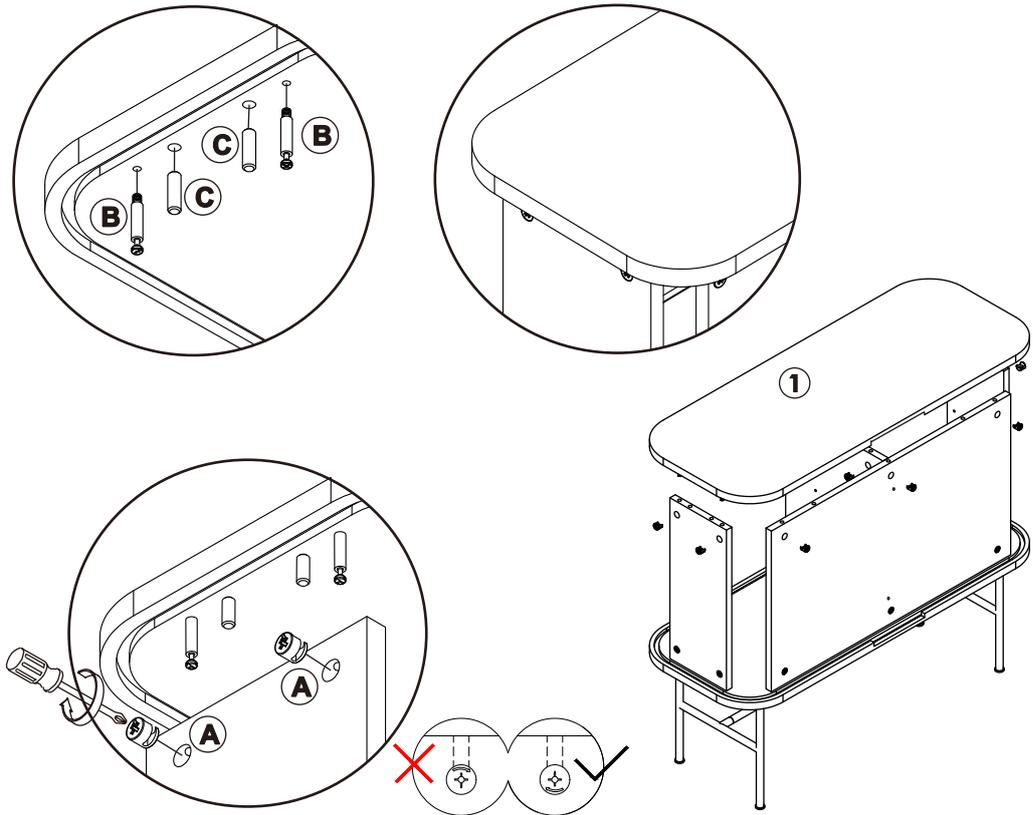
Use Minifix Housing(A), Minifix Bolt(B) and Wood Dowel(C) to connect Top Panel (1) with unit together with screw driver (not included).
