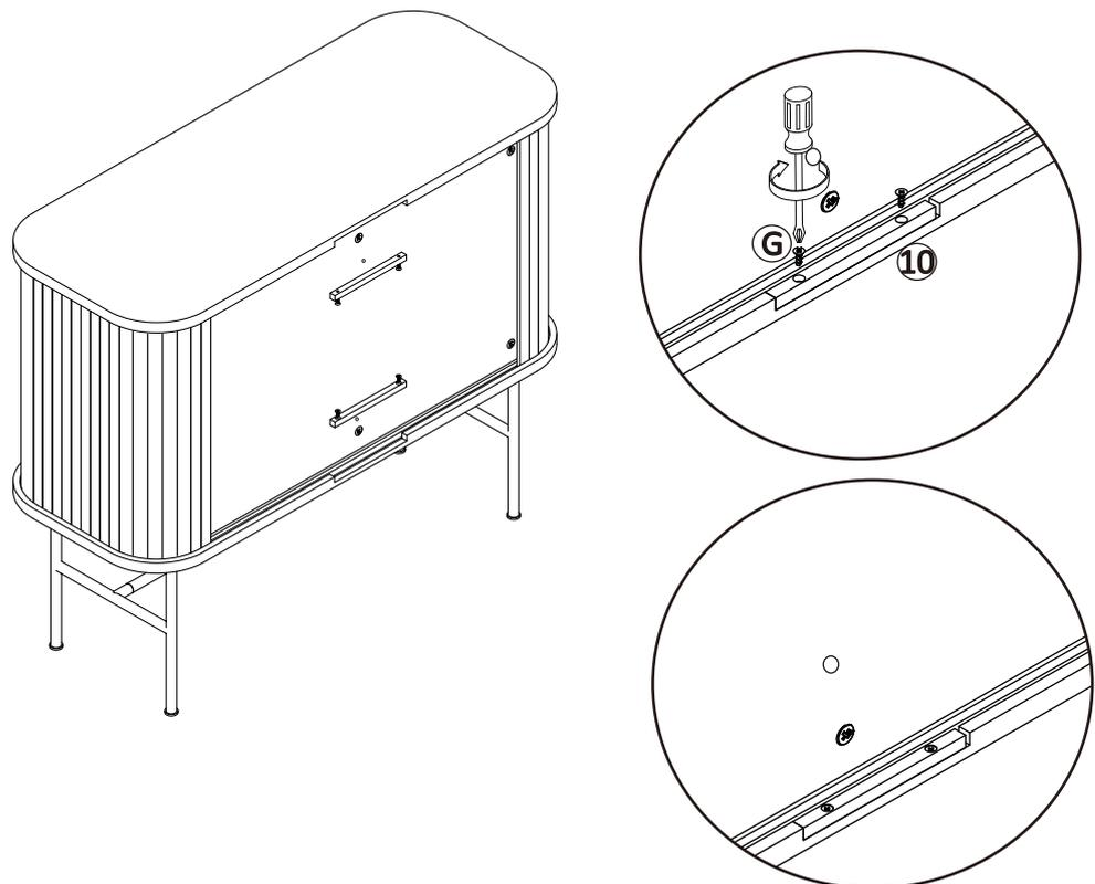
Use JF screw(G) to Connect Groove Cover(10) Tighten with Screw driver (not included)
