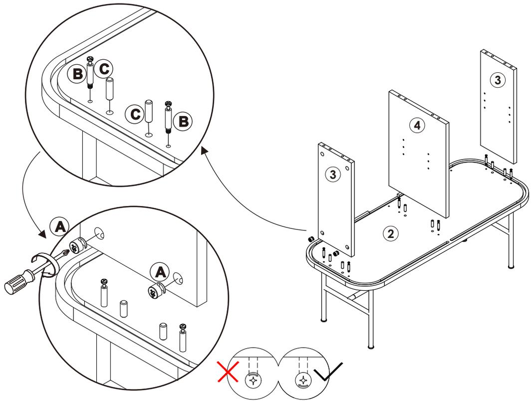
Use Minifix Housing(A) Minifix Bolt(B) and Wood Dowel(C) to connect Side Panel (3) ,Center Panel (4) with Bottom Panel(2) together with screw driver (not included).
