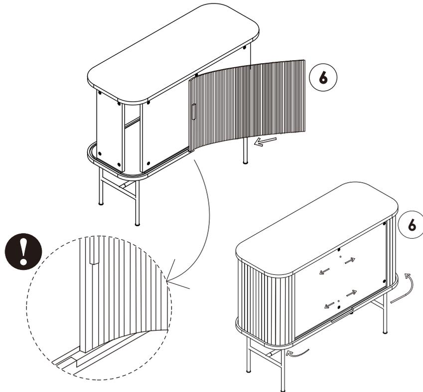
Insert Door Panel(6) into the groove and Slide the Door to the Front
