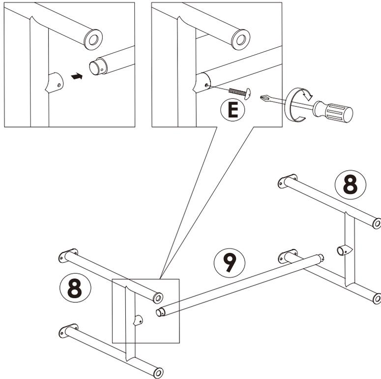
Place Metal Stretcher (9) into Metal Leg (8). Tighten the JMT screw (E) using Screw Driver (not included)
