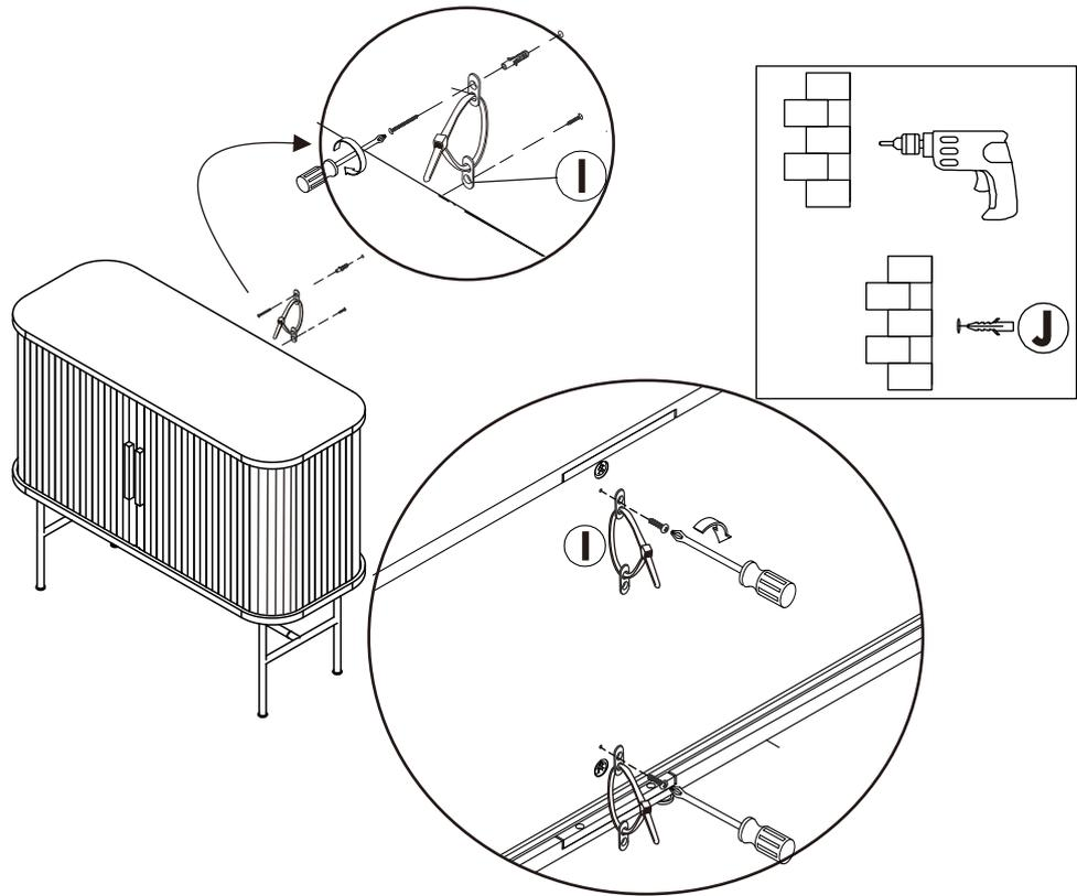
Attach Anti Tipping (I) At Back of the Cabinet. This item should be attached to the wall. **(It is important to sink your screws into a wall stud or use drywall anchor.)**
